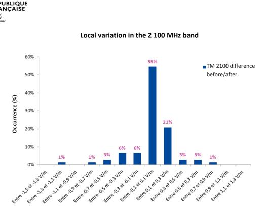
Figure 12. Distribution of differences between 2 100 MHz band contribution before and after 5G roll out at 772 100 MHz sites
