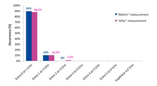
Figure 11. Distribution of exposure levels in the2 100 MHz band before and after 5G roll out at 77 2 100 MHz sites
