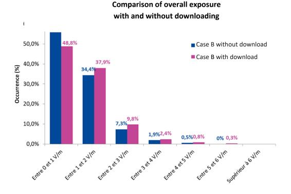
Figure 22. Distribution of the average level over 6 minutes from the specific measurement with 5G solicitation included in the case B overall exposure by calculation, and compared to the case B measurement "after" without specific network solicitation
