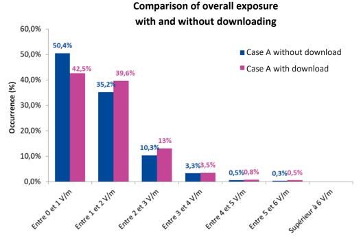
Figure 21. Distribution of the average level over 6 minutes from the specific measurement with 5G solicitation included in case A global exposure by calculation, and compared to the case A measurement "after" without specific network solicitation
