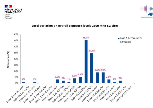
Figure 14. Distribution of differences between overall exposure levels before and after 5G roll out on 102 5G sites in the 2 100 MHz band
