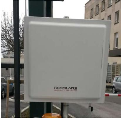
L'objet de l'analyse spectrale est de vérifier le respect des limites de rayonnements fixées par la norme harmonisée ETSI EN 302-208-1 V2.1.2 "*Electromagnetic compatibility and Radio spectrum Matters (ERM); Radio Frequency Identification Equipment operating in the band 865 MHz to 868 MHz with power levels up to 2 W and in the band 915 MHz to 921 MHz with power levels up to 4 W*".
