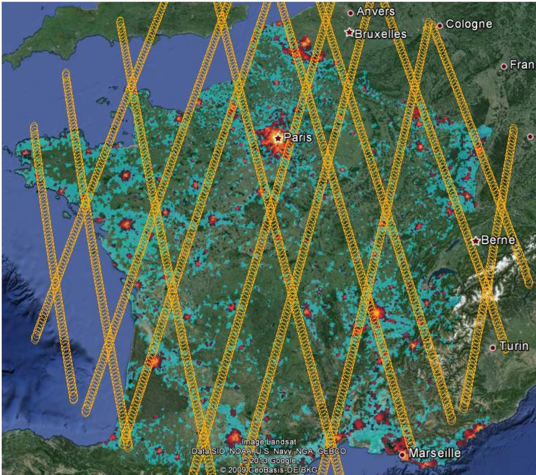
Figure 2: Active RLAN deployment (blue and red surface in the case of 0.04 AR/inh (Around 2 640 000 ARs) and only red surface in the case of 0.004 AR/inh (Around 264 000 ARs) and satellite positions (orange circle) during 15 days
