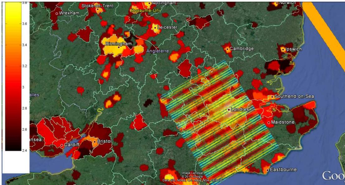
Figure 6: Active RLAN deployment for 0.004 AR/inh, satellite positions (orange line) and antenna footprint (every 2 seconds)
