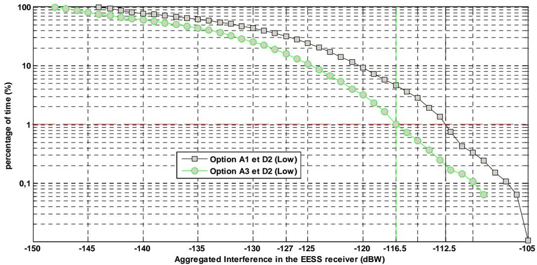
Figure 8: Comparison between each antenna option (A1 & A3) for French territory. Simulations are performed with 0.004 AR/inh (D2 Low).
