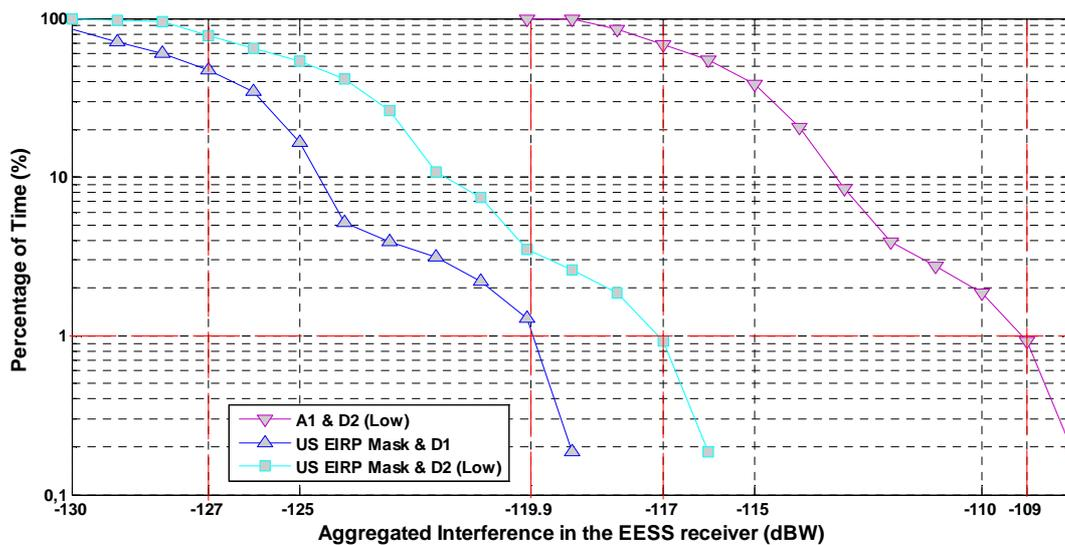
**Figure 9: Comparison between simulations with the US EIRP Mask and two RLAN densities (D1 & D2) over London area.**
