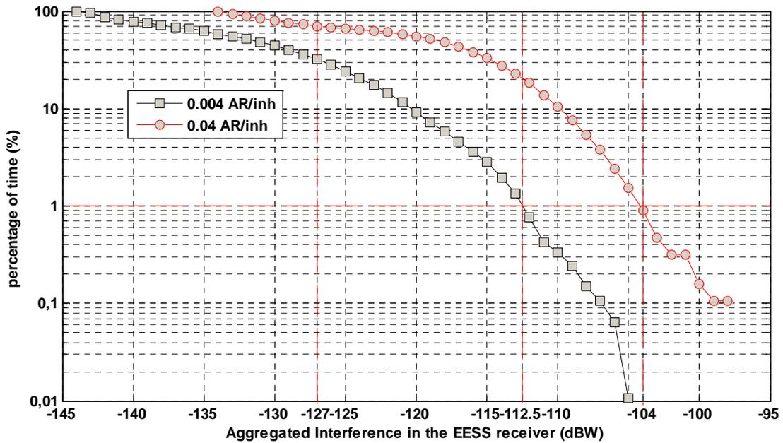
Figure 3: simulation results of CDF for 0.004 & 0.04 AR/inh (D2-low and D2-high) deployed in FRANCE
