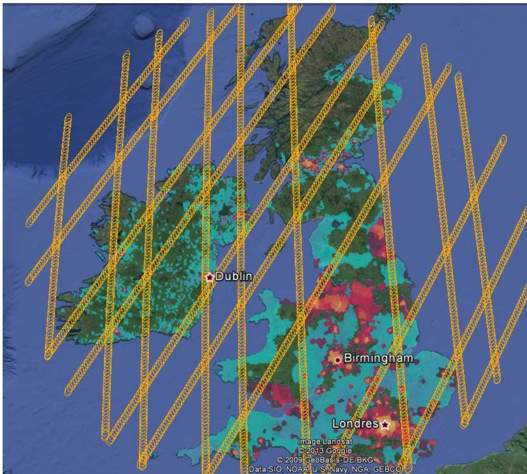
**Figure 4: Active RLAN deployment (blue and red surface in the case of 0.04 AR/inh (Around 2 400 000 ARs for UK and 160 000 for Ireland) and only red surface in the case of 0.004 AR/inh (Around 240 000 ARs for UK and 16 000 for Ireland)) and satellite positions (orange circle) during 15 days**
