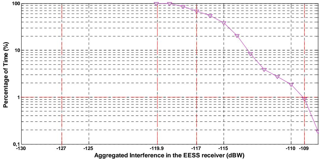
Figure 7: simulation results of CDF for 0.004 AR/inh (D2-low) for one passage of the satellite over great London. The simulation results presented in Figure 6 clearly show that the EESS protection criterion is exceeded by 18 dB for 0.004 active RLAN per inhabitant over great London.
