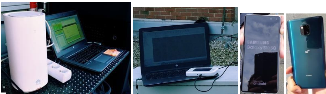
Figure 3: Different equipment used as receivers on 5G pilots. From left to right, a CPE "customer premises equipment", a 5G modem and two 5G mobiles.
