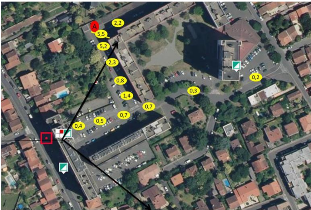
Figure 12: Satellite view of the Toulouse site with the position of the CPE in red and the field strengths measured in V/m at different points in yellow for a continuous emission over 100 MHz bandwidth with a maximum power of 200 W.
