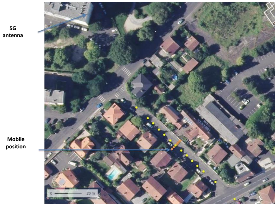
Figure 16: Aerial view of the Pau site with the antennas on a building 45 m high and the CPE located 125 metres from the antenna, in direct view in a street at the foot of the building supporting the antennas. The yellow and orange dots are the measuring points.
