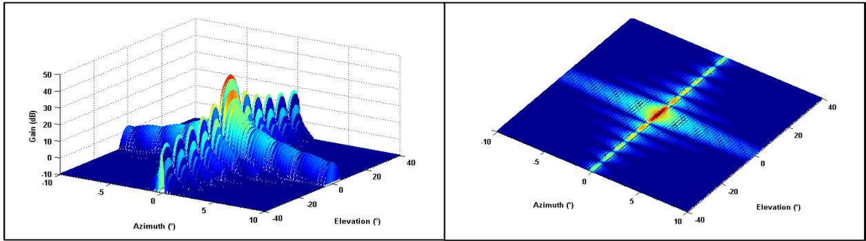
**Figure 1: Antenna gain representation of EESS satellite (Sentinel-1). 3D representation (left) and projection on a plan (right)**
