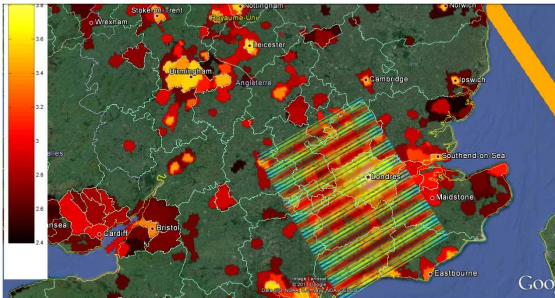
Figure 6: Active RLAN deployment for 0.004 AR/inh, satellite positions (orange line) and antenna footprint (every 2 seconds)
