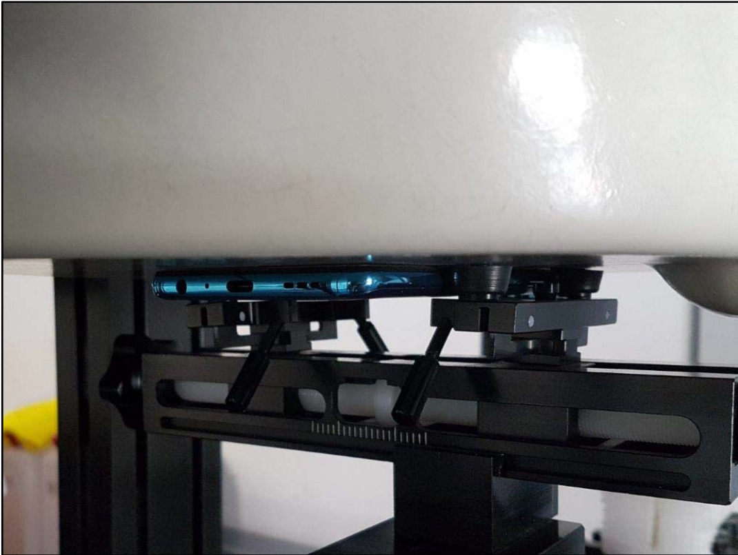
Photo 17: Test position body worn front side with 0 mm distance
