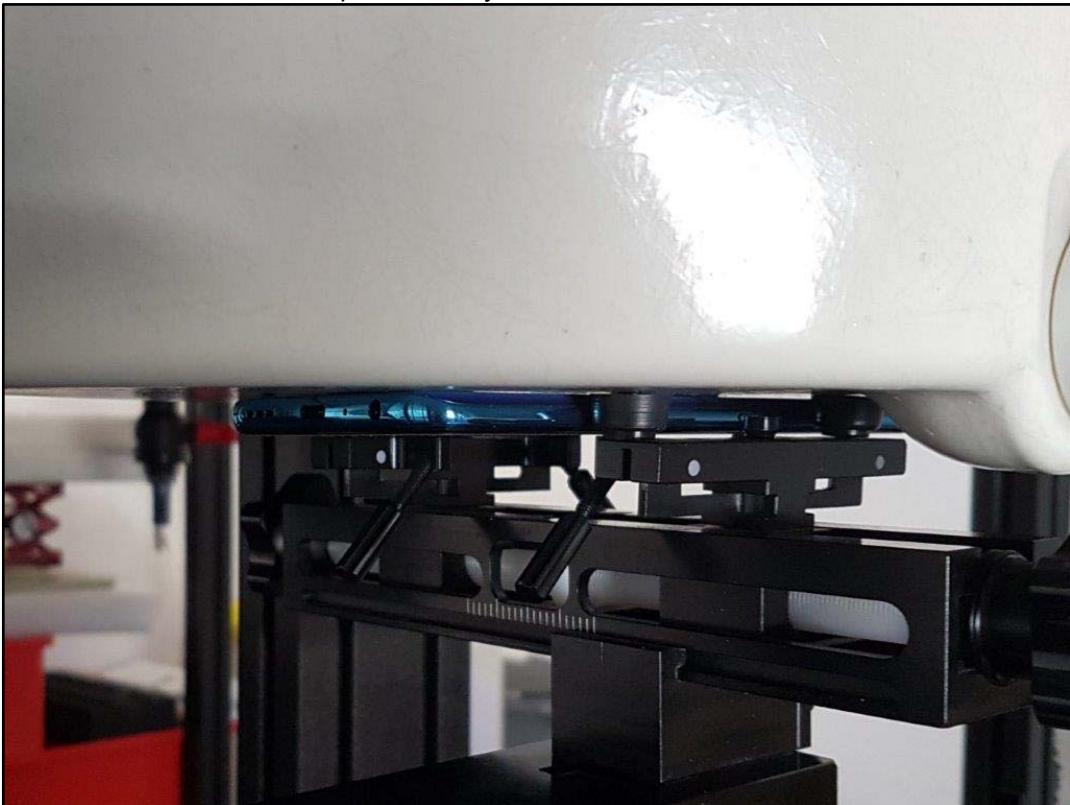
Photo 18: Test position body worn back side with 0 mm distance
