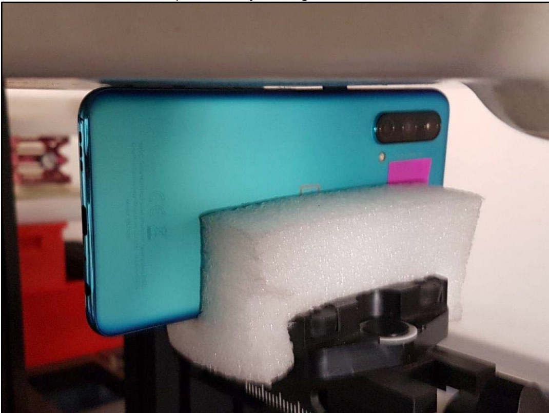
Photo 20: Test position body worn right side with 0 mm distance
