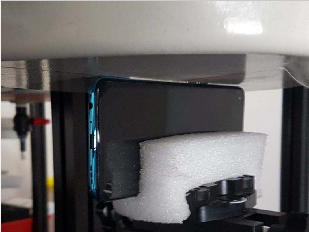
Photo 20: Test position body worn right side with 0 mm distance
