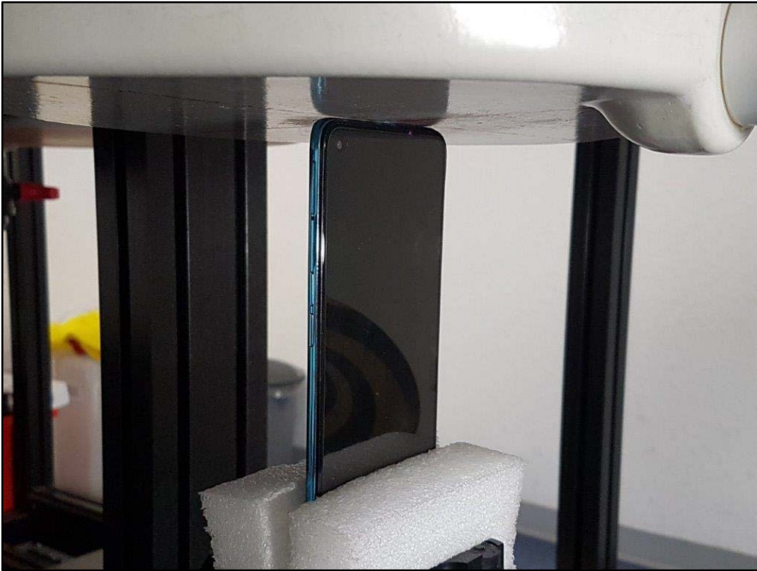
Photo 22: Test position body worn bottom side with 0 mm distance
