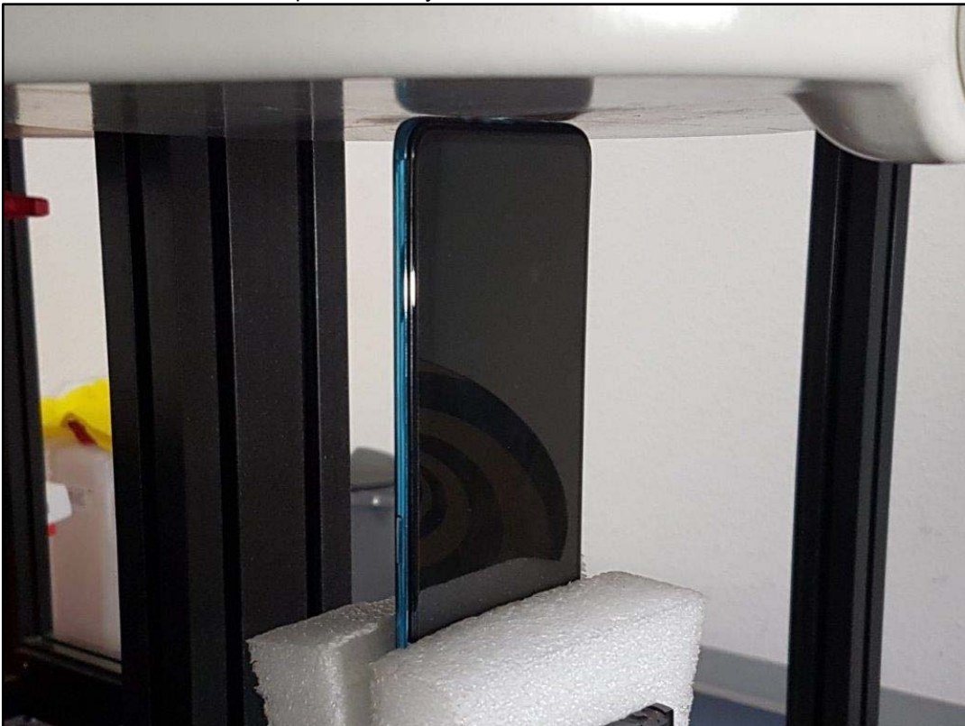
Photo 22: Test position body worn bottom side with 0 mm distance
