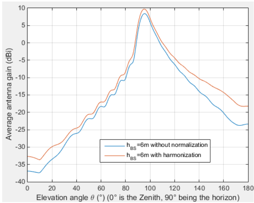
FIGURE 25 Average gain (BS mechanical tilt=10°)
